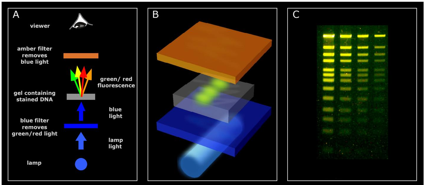
**Figure 2. The Dark Reader optical system.** (A, B) Optical components and relevant light paths of the Dark Reader design. (C) DNA samples separated by agarose gel electrophoresis, stained with SYBR Green and viewed on a Dark Reader transilluminator. The image was recorded with a CCD camera.
